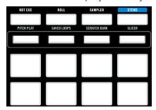
**HOT CUE mode:** Pads 1-8 trigger Serato DJ Pro Cue points, and if no Cue point is present on that slot/pad, pressing that pad will set a Cue point. Holding down the **SHIFT** button while pressing a populated pad will delete the Cue point from the respective pad/slot. If Serato Flip is activated: Parameter 1 left engages Flip Record, while right starts your Flip, and holding **SHIFT** means left is Flip Loop while right is Flip on/off.
